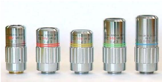
Plane-apochromatic incident light objectives with extra long working distances (RMS thread, parfocalizing length = 95 mm)
